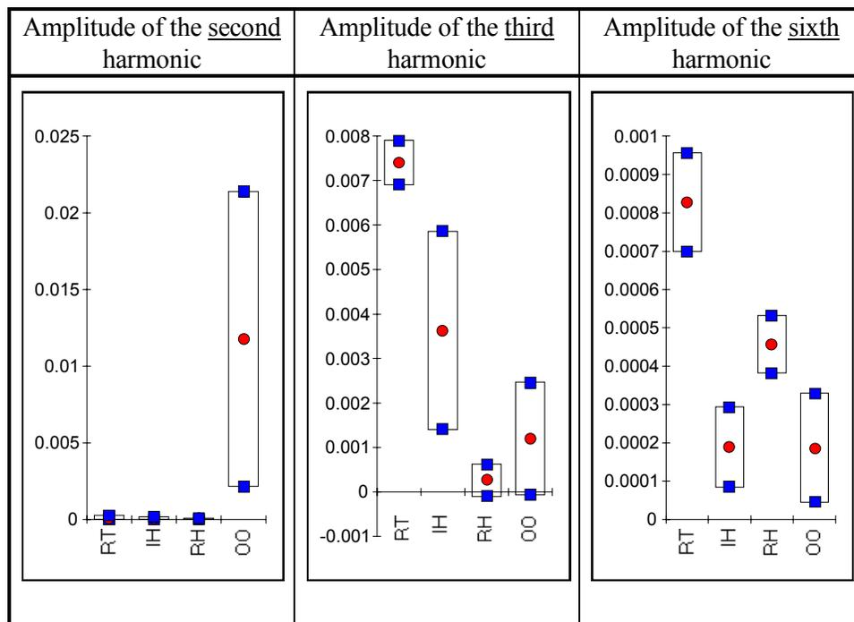
**Figure 2.** Average values of the amplitude and standard deviation of the second, third and sixth harmonics for the four different types of silver halide crystals (RT - triangles, IH - irregular hexagons, RH - hexagons, OO - overlapping crystals).
