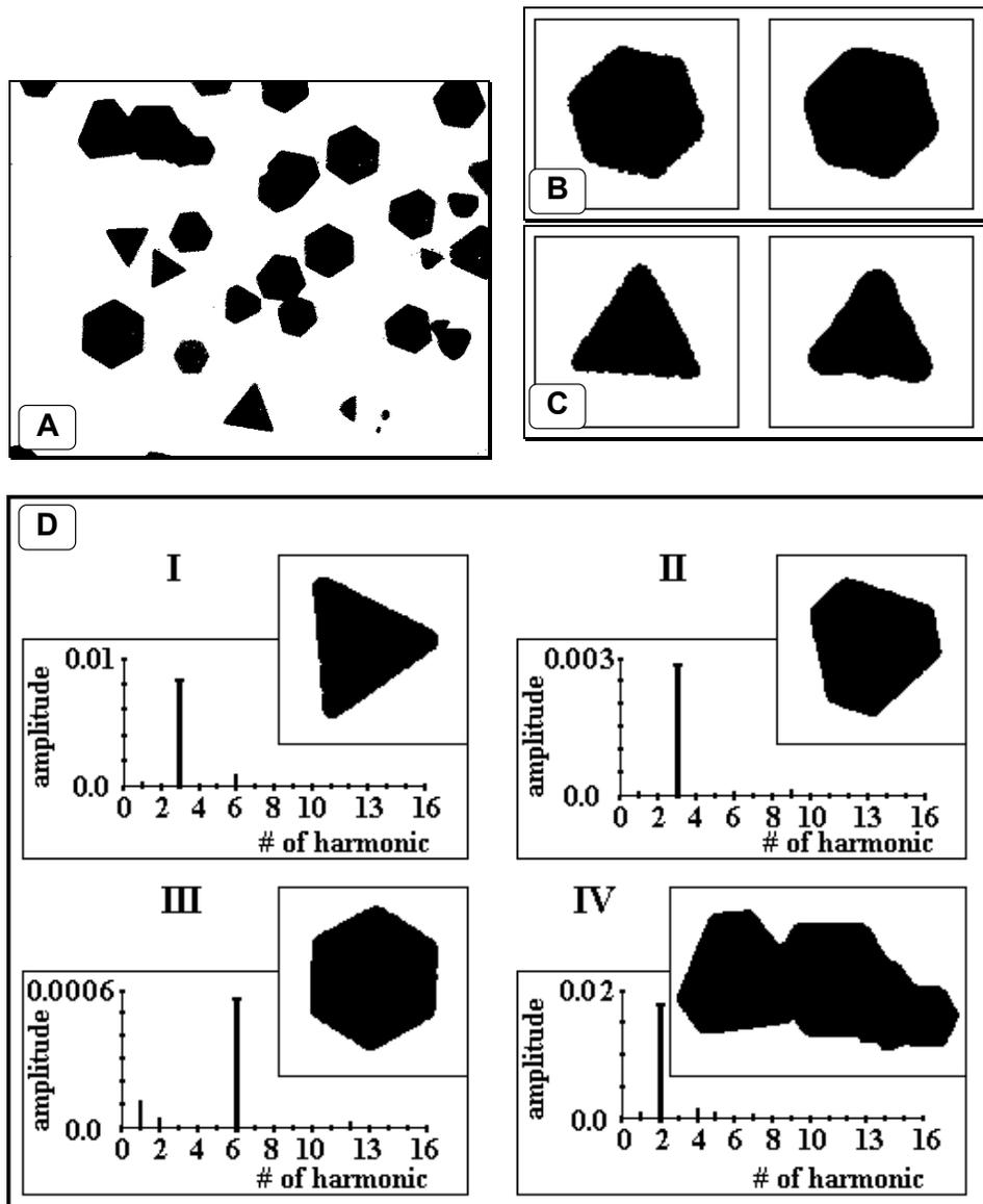
**Figure 1.** A. 'T-grain' silver halide crystals (SEM backscattered electron image); B. The hexagonally shaped silver halide crystal (left) and restored hexagon by using the first 6 Fourier coefficients (right); C. The triangular silver halide crystal (left) and restored triangle by using the first 6 Fourier coefficients (right); D. Amplitude of the Fourier coefficients for different crystal shape.
