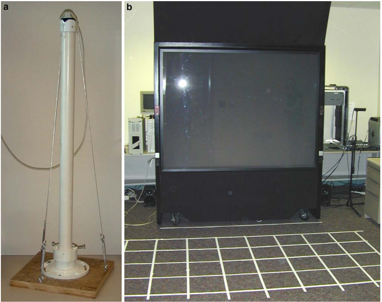
Fig. 1 Calibration table acquisition device used in this study. Two-dimensional grid (b) is laid on the floor in front of the I-Desk; sensor holder (a) is moved on the grid
